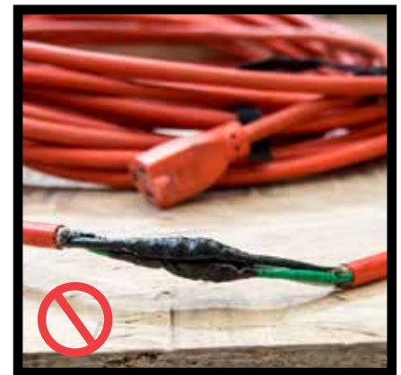
Do not use damaged cords. No usar cables dañados.
